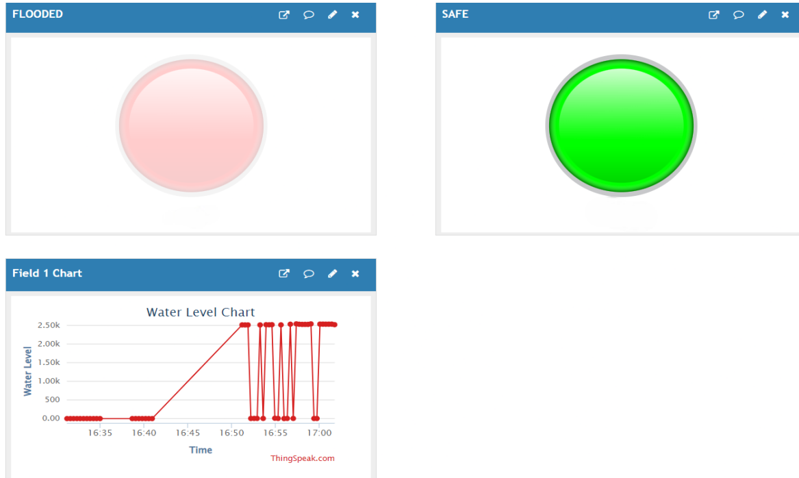
Figure 4: Visualization of water level on ThingSpeak cloud platform
